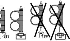
Install saddles directly to cleat or anchor bar (washers & nut), no visible tread.
